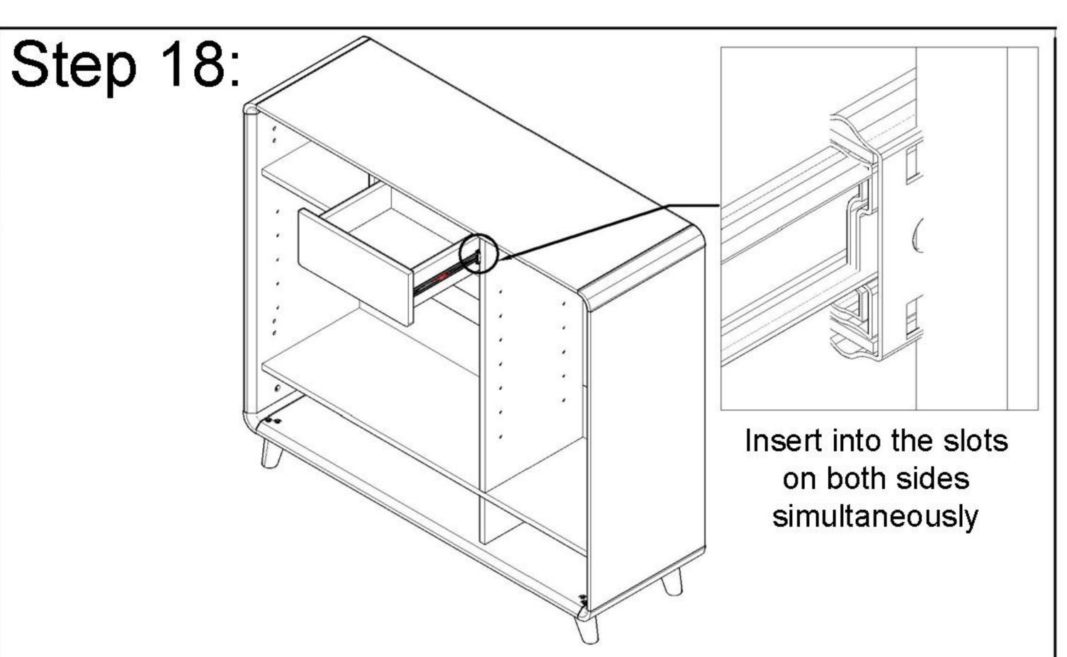
Pull the G part fixed to panels 6 and 7 to its full length, with the silver ball-bearing section at the front. Insert the small tracks on both sides of the drawer into the slots, then gently push to secure.
