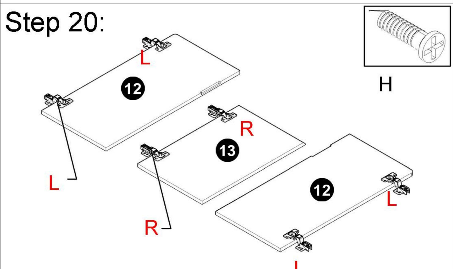
Note: When installing L or R, if you encounter resistance while tightening the screws, stop immediately. Continuing to apply force may cause the threads to strip or damage the mechanism.
