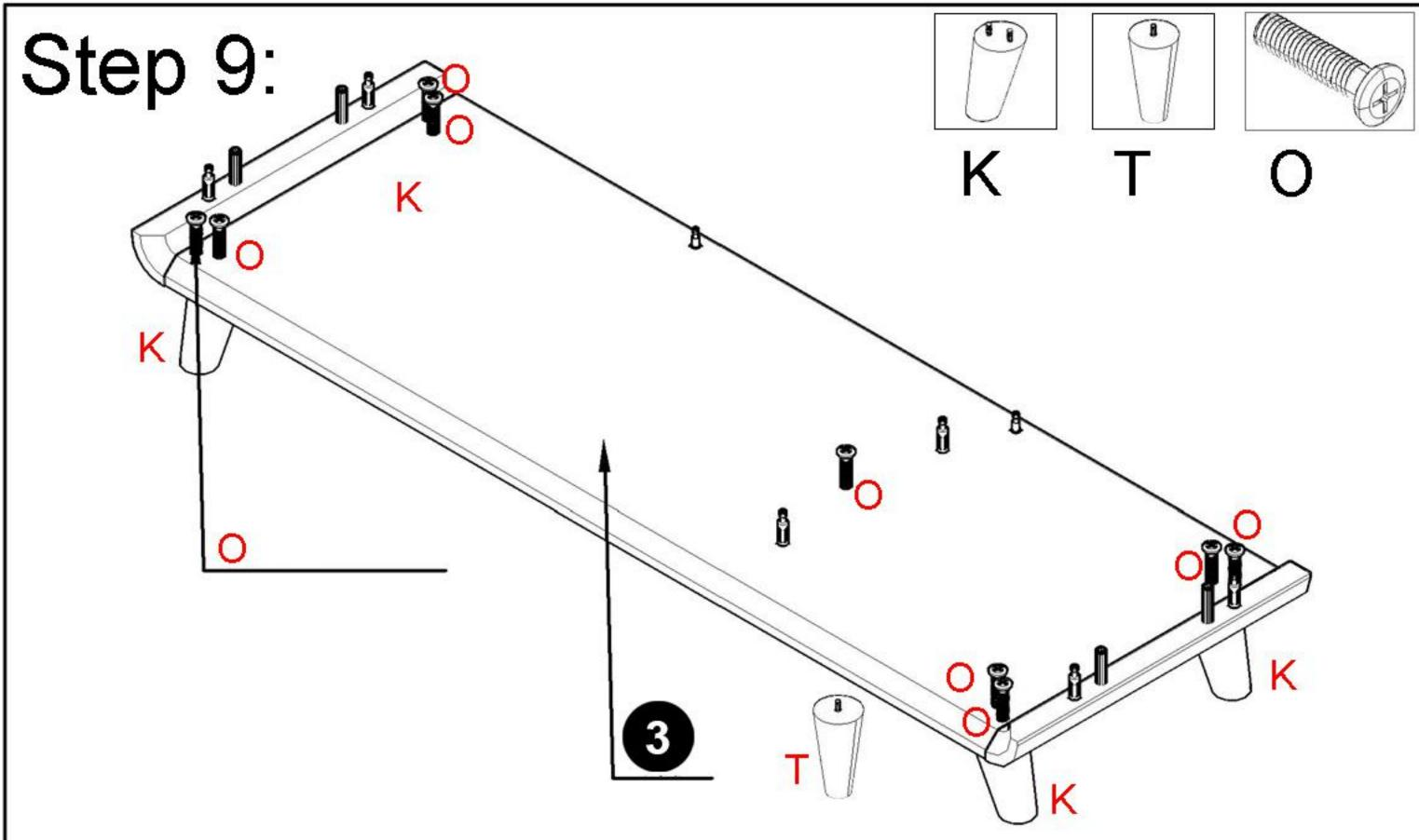
Install K and T to the underside of panel 3 using screws O
