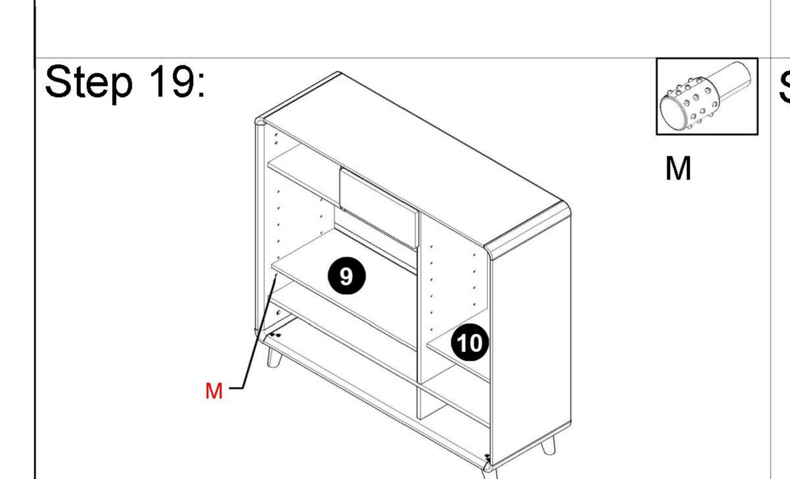
Install M onto panels 4 and 7, then place panels 9 and 10 onto M
