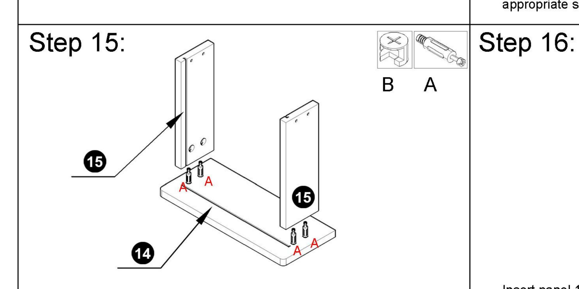
Note: The grooves on panel 15 must align with the grooves on panel 14, and secure all joints with B
