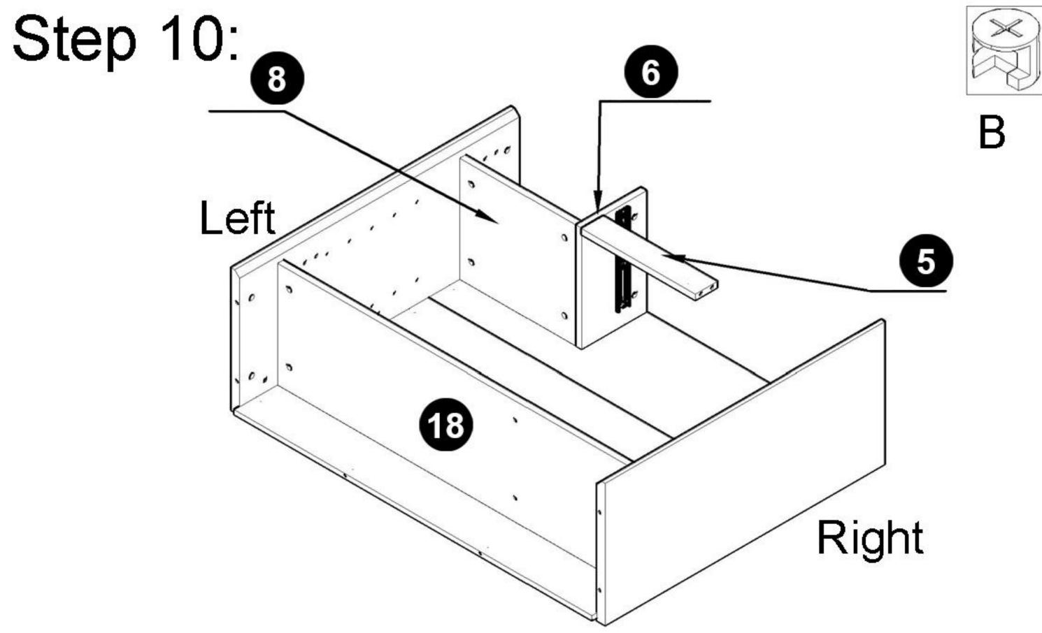
Join the corresponding holes of steps 6, 8, 6, and panel 5, and secure with B
