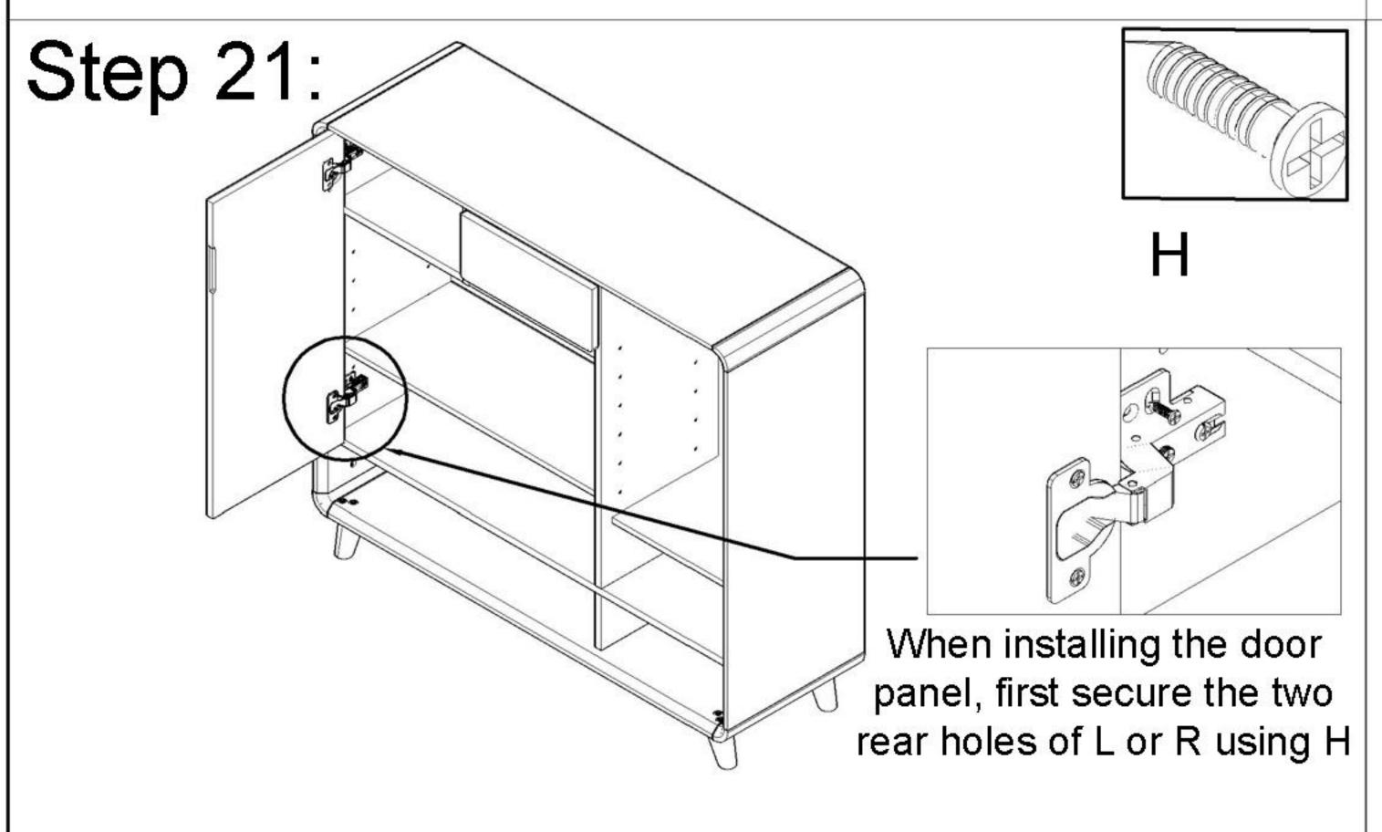
First, secure the rear two holes of L or R with H, then install the front two holes. Refer to the initial hinge installation instructions to adjust the door's height and gap.
