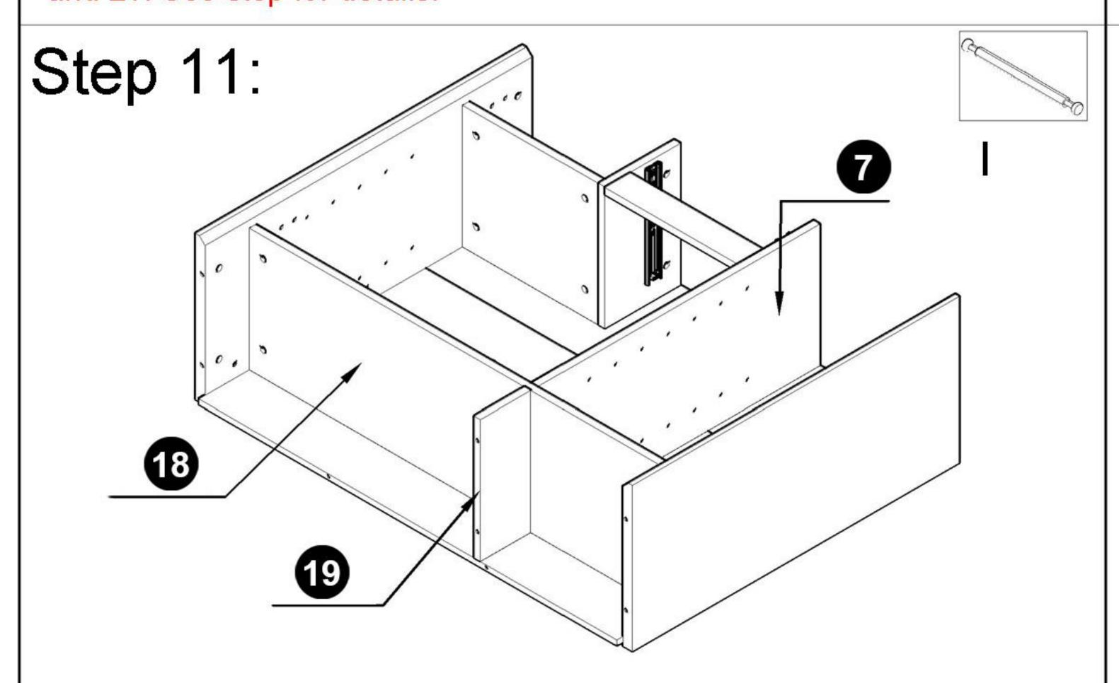
Connect panel 7 to panel 5. Attach the bottom of panel 7 to panels 18 and 19 with connector I, and secure all joints with B
