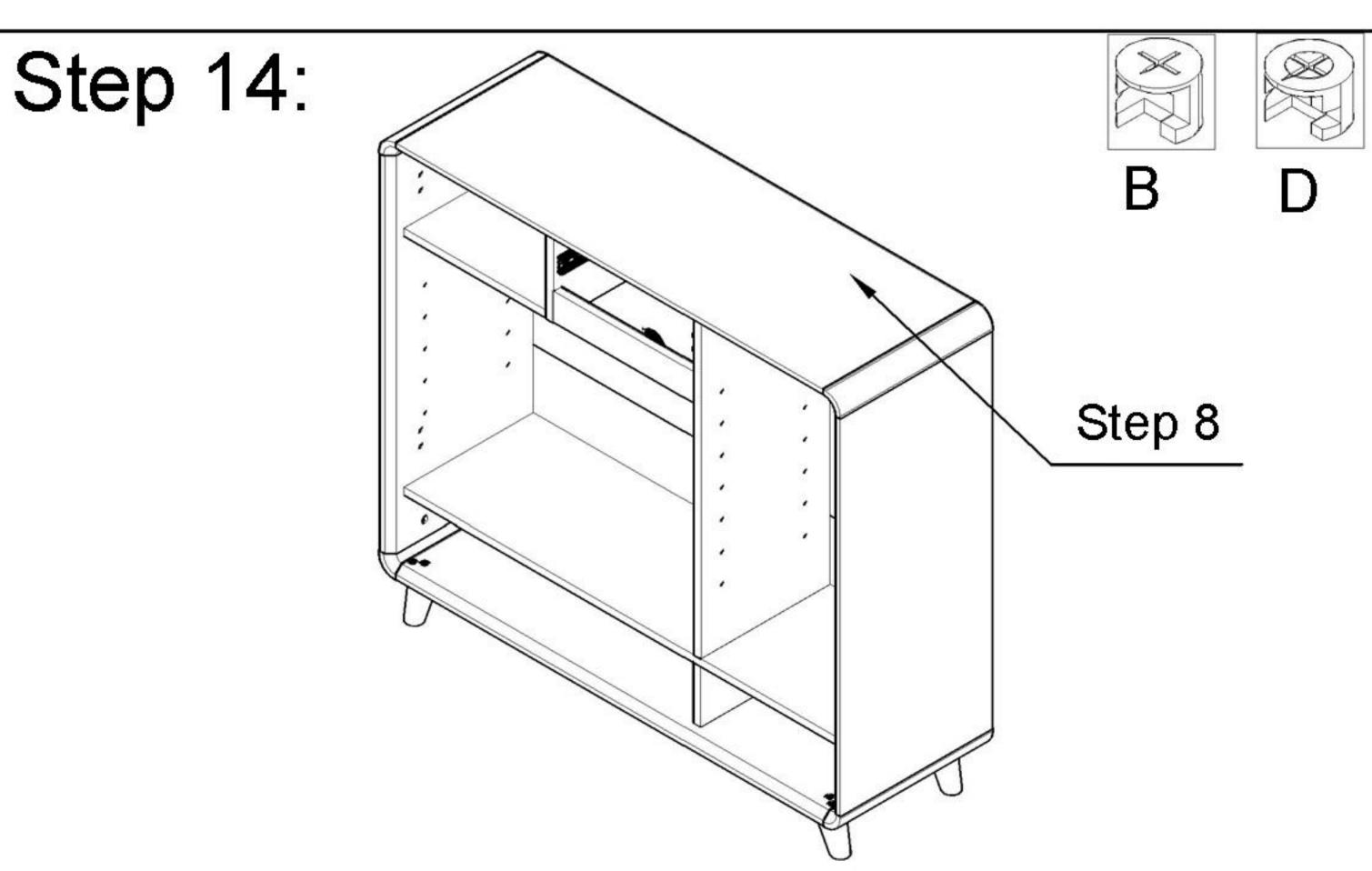
Connect steps 8 and 13, and secure the connections with the appropriate size D or B
