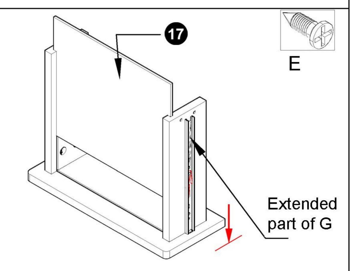
Insert panel 17 as indicated by the arrow. Position the extended part of G on the outside of both panel 15 pieces. Ensure the stopper side of G rests against panel 14
