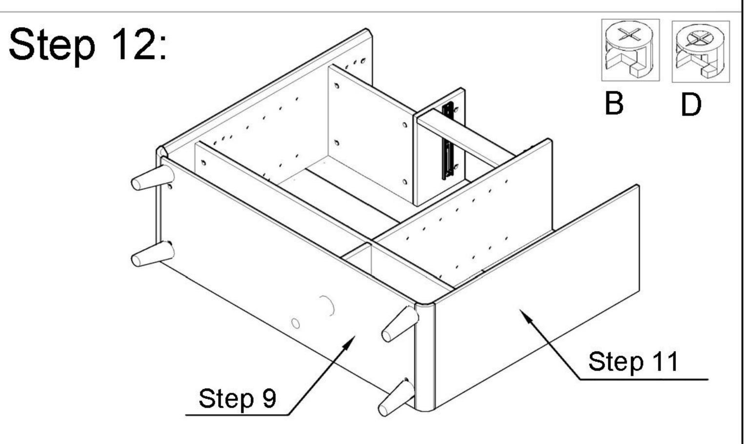
Connect steps 9 and 11, and secure the connections with the appropriate size D or B
