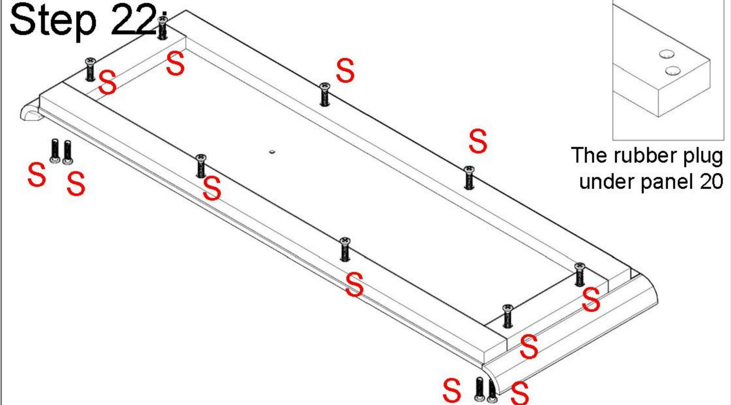
If cabinet legs are not required, proceed with the installation of the floor skirting board by following the instructions below. First, use S to pass through the bottom panel hole and secure it in the rubber plug holes of panels 19 and 20. Then, use S to pass through panels 19 and 20 to secure the rubber plug holes of the bottom panel. The screw direction is shown in the diagram. Please pay attention to the screw installation direction.
