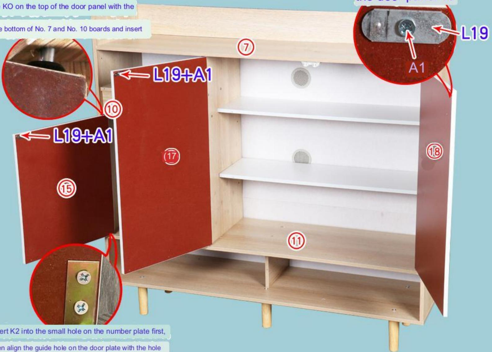
2. Insert K2 into the small hole on the number plate first, then align the guide hole on the door plate with the hole of K2 and fix it with A1 first. After the door plate is adjusted,
