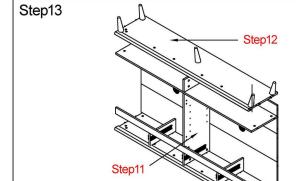
Connect the assembly from Step 12 to that from Step 11, and fasten using part A or D.
