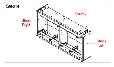
Connect steps 13 and 3 Left + Right, and fasten using part A or D.
