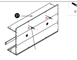
Insert part K through the back of part 20 to secure part 21.
