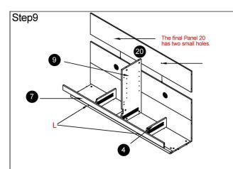
After installing part 20, use part A to secure all panels.
