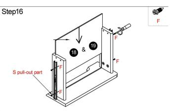
Insert the correctly sized bottom panel (18 or 19) into the groove. Use part F to install the S pull-out part.
