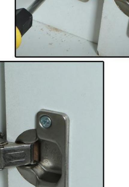
As shown in the picture, loosen the screw pointed
