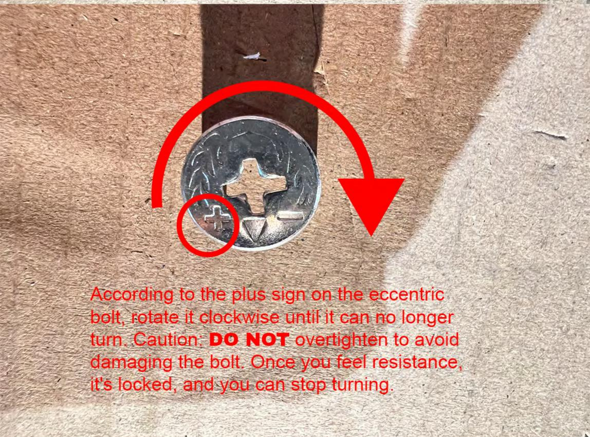
According to the plus sign on the eccentric bolt, rotate it clockwise until it can no longer turn. Caution: **DO NOT** overtighten to avoid damaging the bolt. Once you feel resistance, it's locked, and you can stop turning.
