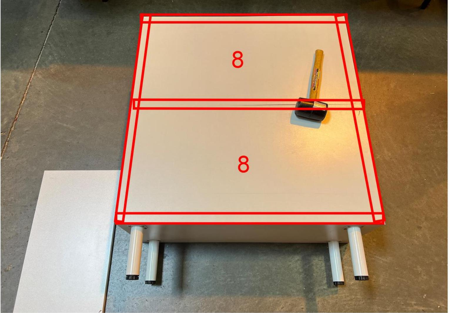
Place 8(the back panel) in the correct position, fully covering the back side of the cabinet. Make sure to leave enough space along the edges for proper fastening by H. 8 x 2 should be installed using the same procedure. (Hammer not included.)
