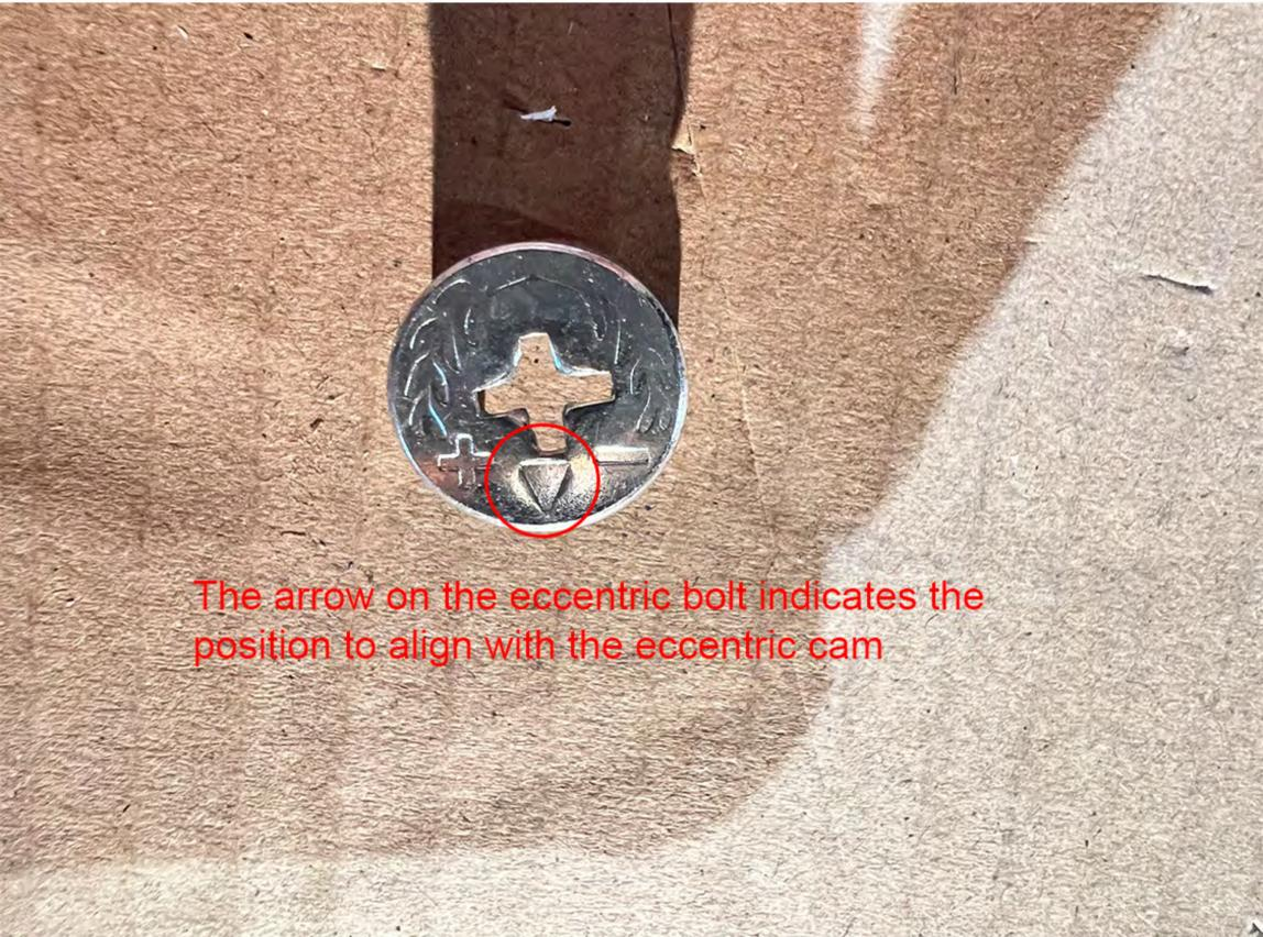
The arrow on the eccentric bolt indicates the position to align with the eccentric cam
