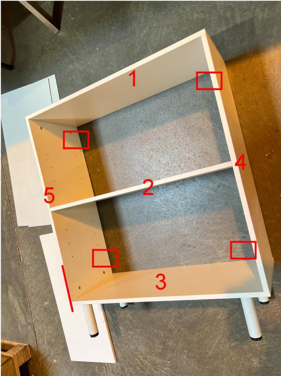
Use part G to fix part A under panel 3. There are no holes, so you need to screw it in yourself. Place A where you want it. A drill is recommended (not included).
