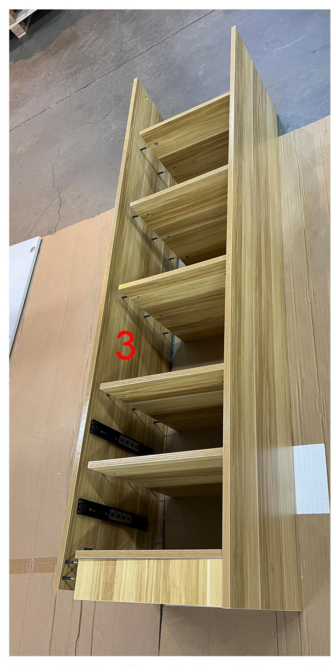
After joining Panels 3 and 4, use F to securely tighten all the round pre-drilled holes. Don't forget the cabinet bottom.
