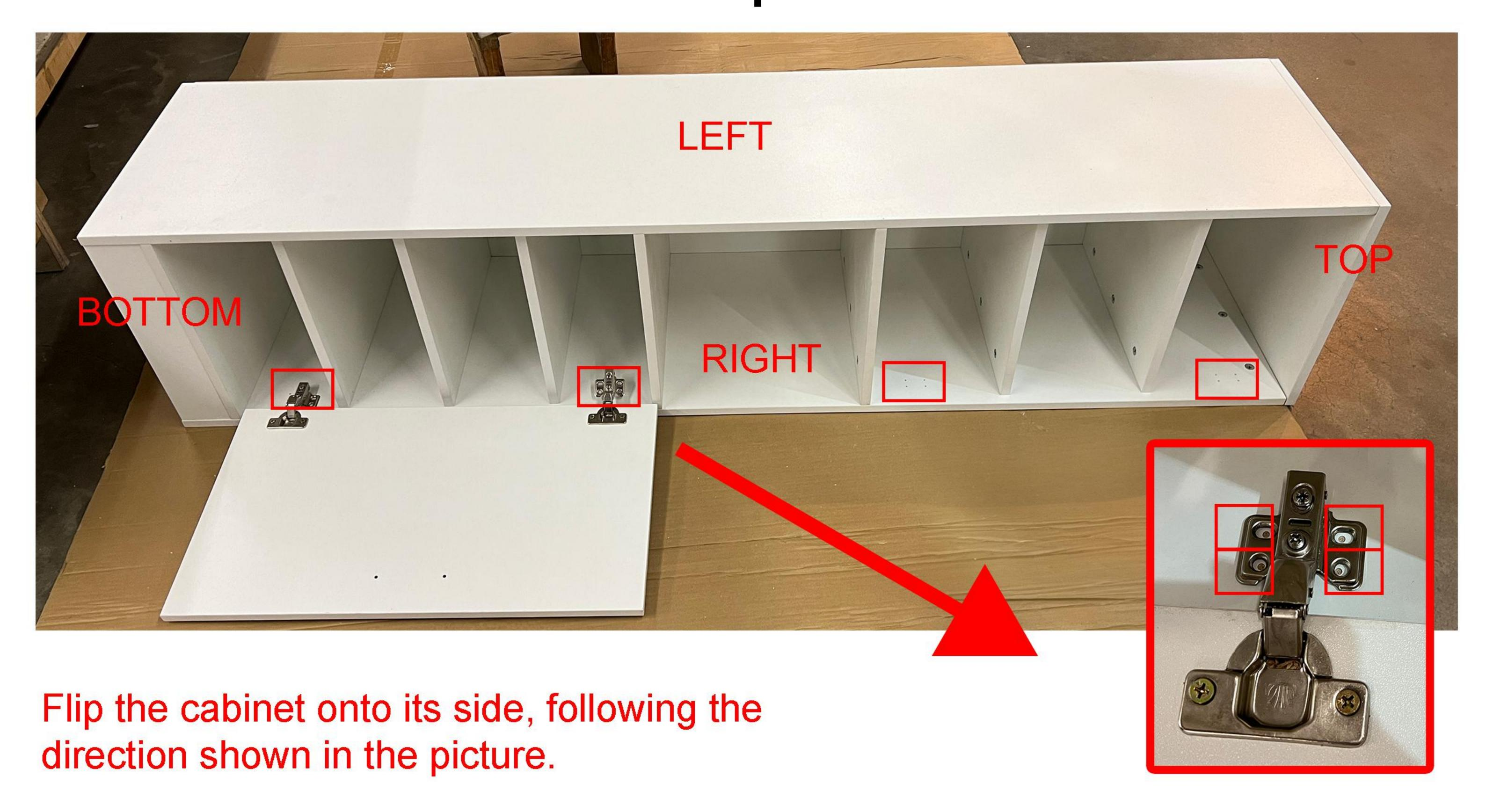
Pay attention to the pre-drilled holes on the right side of the cabinet. Connect the other side of G from Step 1 to the cabinet using B.
