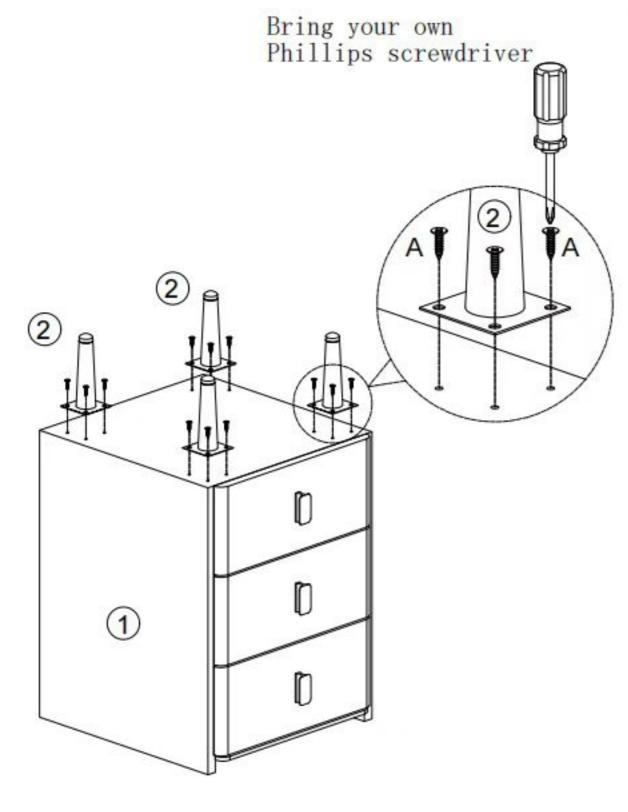
Note: After unpacking, please check the number of assembled parts as shown in the picture against the instruction manual first to see if it is correct. As shown in the picture, use a Phillips screwdriver to fix part 2 with hardware A on the bottom of part 1.
