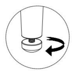
If the cabinet is not level when placed, adjust the bottom feet as shown until level.
