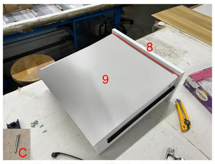
Insert Panel 9 into the groove of Panel 8 and secure it using C.
