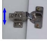
As shown in the figure, loosen the screw that the screwdriver points to, push the lower door panel and hinge upward, and then tighten the screw. Push the upper door panel and hinge downward, and then tighten the screw.
