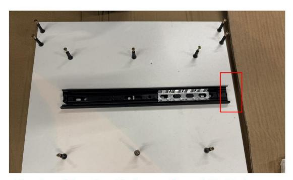
Align the slide rails with the small pre-drilled holes. Position the rails approximately **17mm** from the side.
