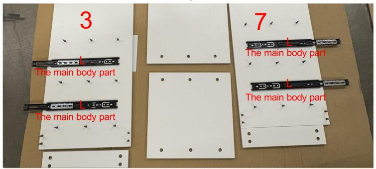
Pay attention to the direction of the sliding rails, ensuring the end with the stopper faces backward. Align the two sliding rails and use B to secure them to the pre-drilled holes. Refer to the marked positions in the diagram for guidance. Ensure the positions of the left and right sliding rails are as parallel as possible.
