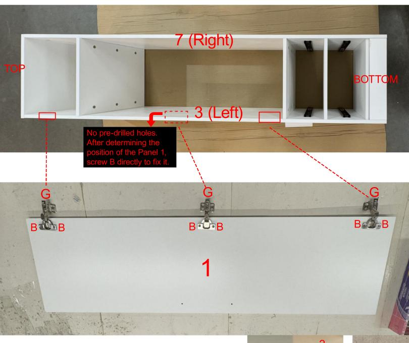
Align the other end of G on Panel 1 with the pre-drilled holes on Panel 3 and secure it using B. For adjusting the door gap, please refer to the initial Instruction for Door Panel Adjustment.
