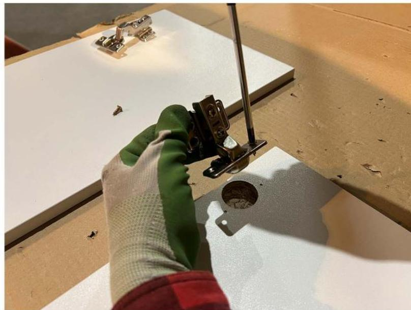
It is recommended not to fully tighten part H at this stage—lightly fasten it first, and fully tighten it at the final step.
