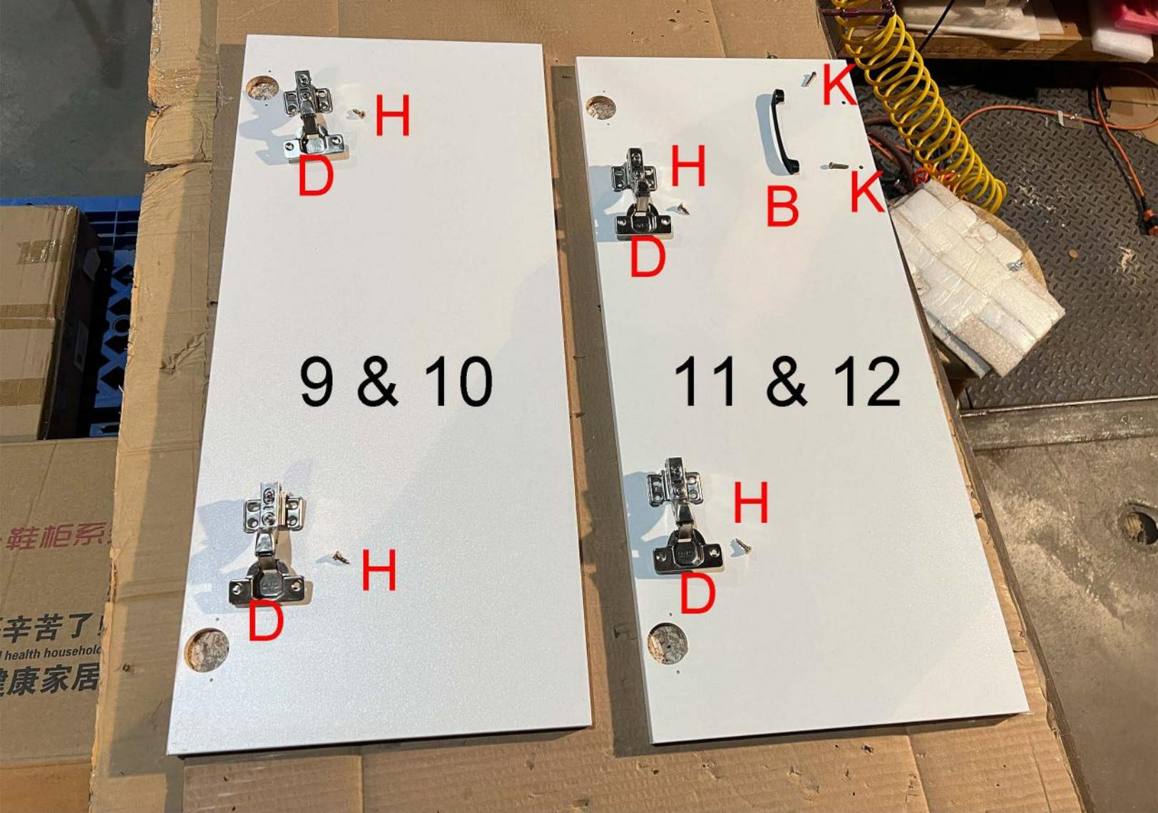
Attach D to Panels 9 – 12 using H.
