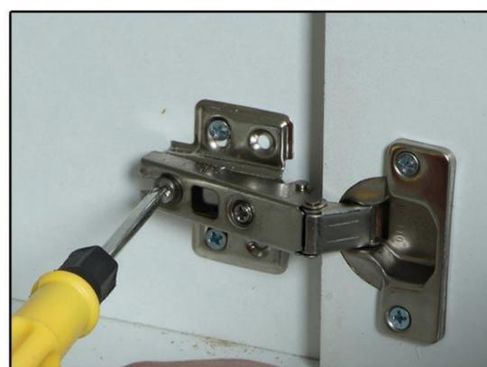
As shown in the picture, loosen the screw pointed by the screwdriver, push the door panel in or pull it out, and then tighten it to solve the above problem.
