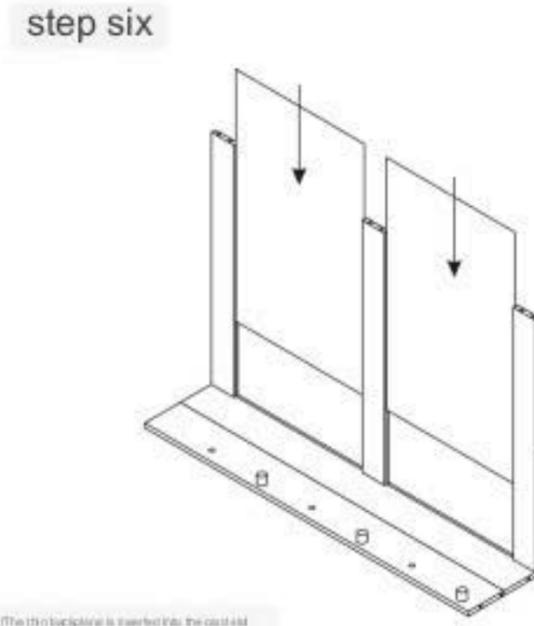
The thin backplate is inserted into the cabinet
