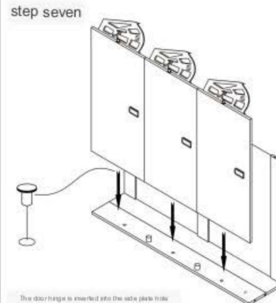
The door hinge is inserted into the side plate hole
