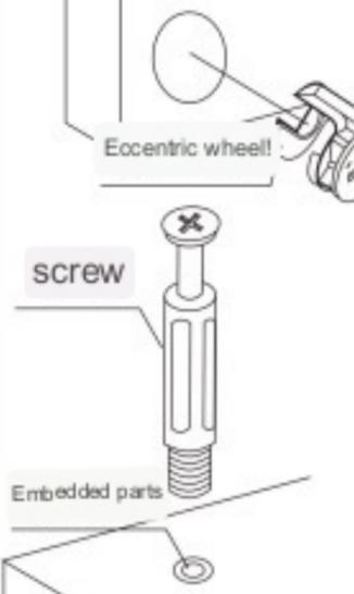
1. Use a hammer or a hard object to knock the embedded part into the hole in the plank (diameter 10mm) to keep the depth consistent with the plank surface
