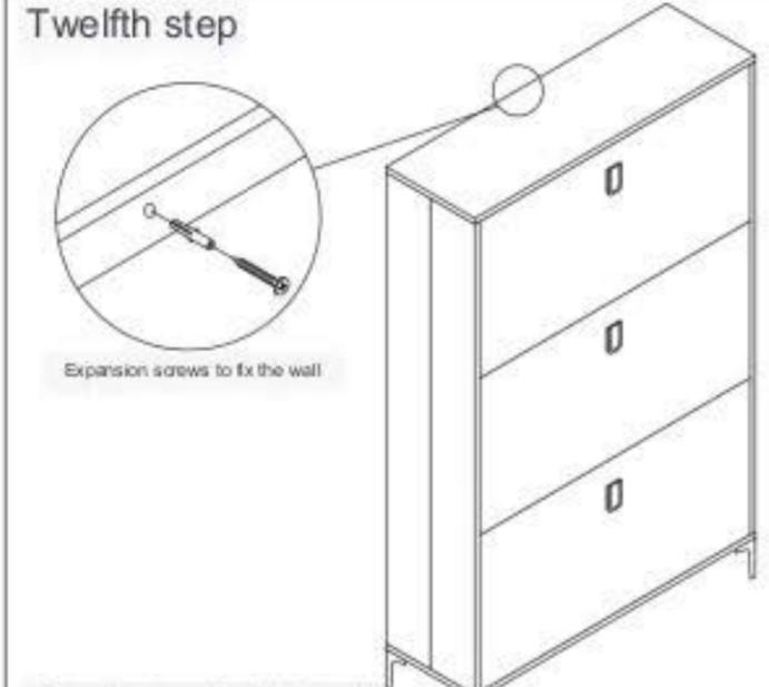
Expansion screws to fix the wall
