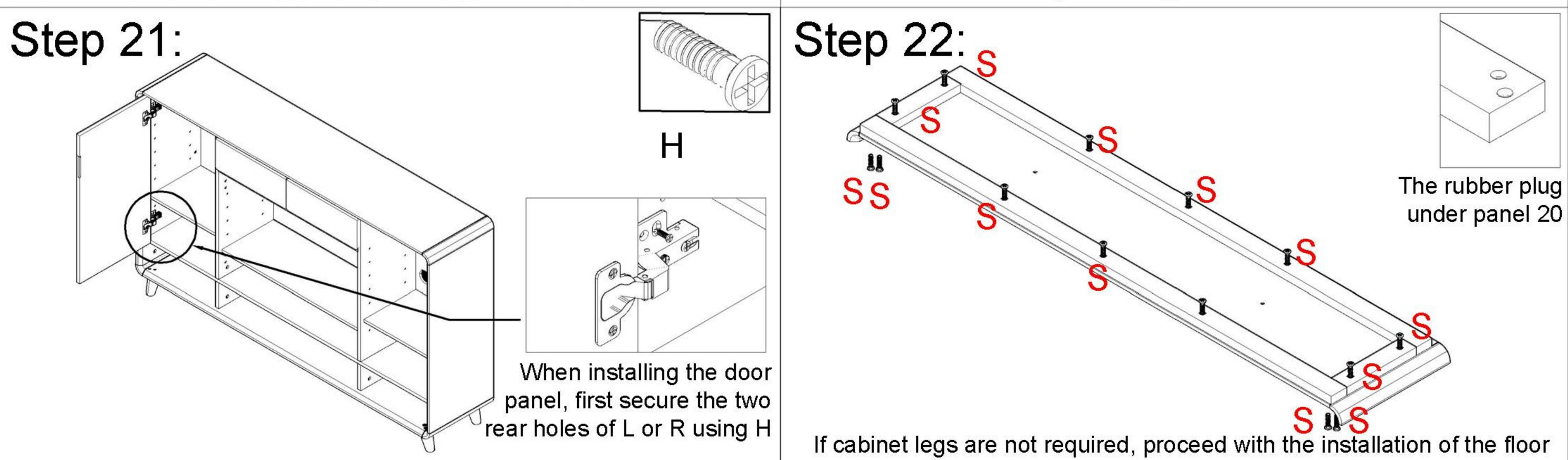
skirting board by following the instructions below. First, use S to pass through the bottom panel hole and secure it in the rubber plug holes of panels 19 and 20. Then, use S to pass through panels 19 and 20 to secure the rubber plug holes of the bottom panel. The screw direction is shown in the diagram. Please pay attention to the screw installation direction.
