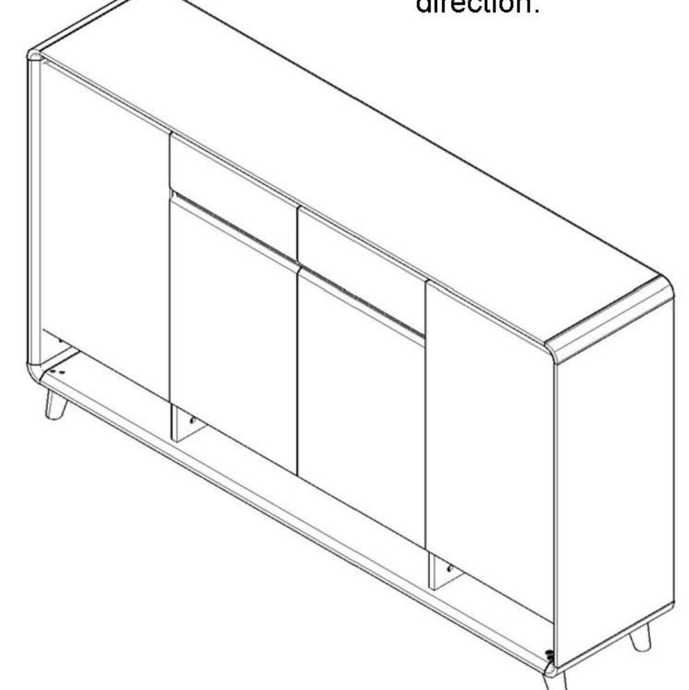
First, secure the rear two holes of L or R with H, then install the front
