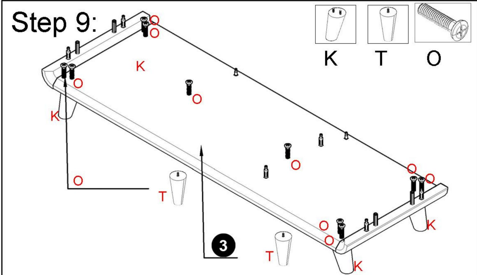
Install K and T to the underside of panel 3 using screws O Note: If you do not wish to install the four cabinet legs, please directly follow the assembly method outlined in Step 22.
