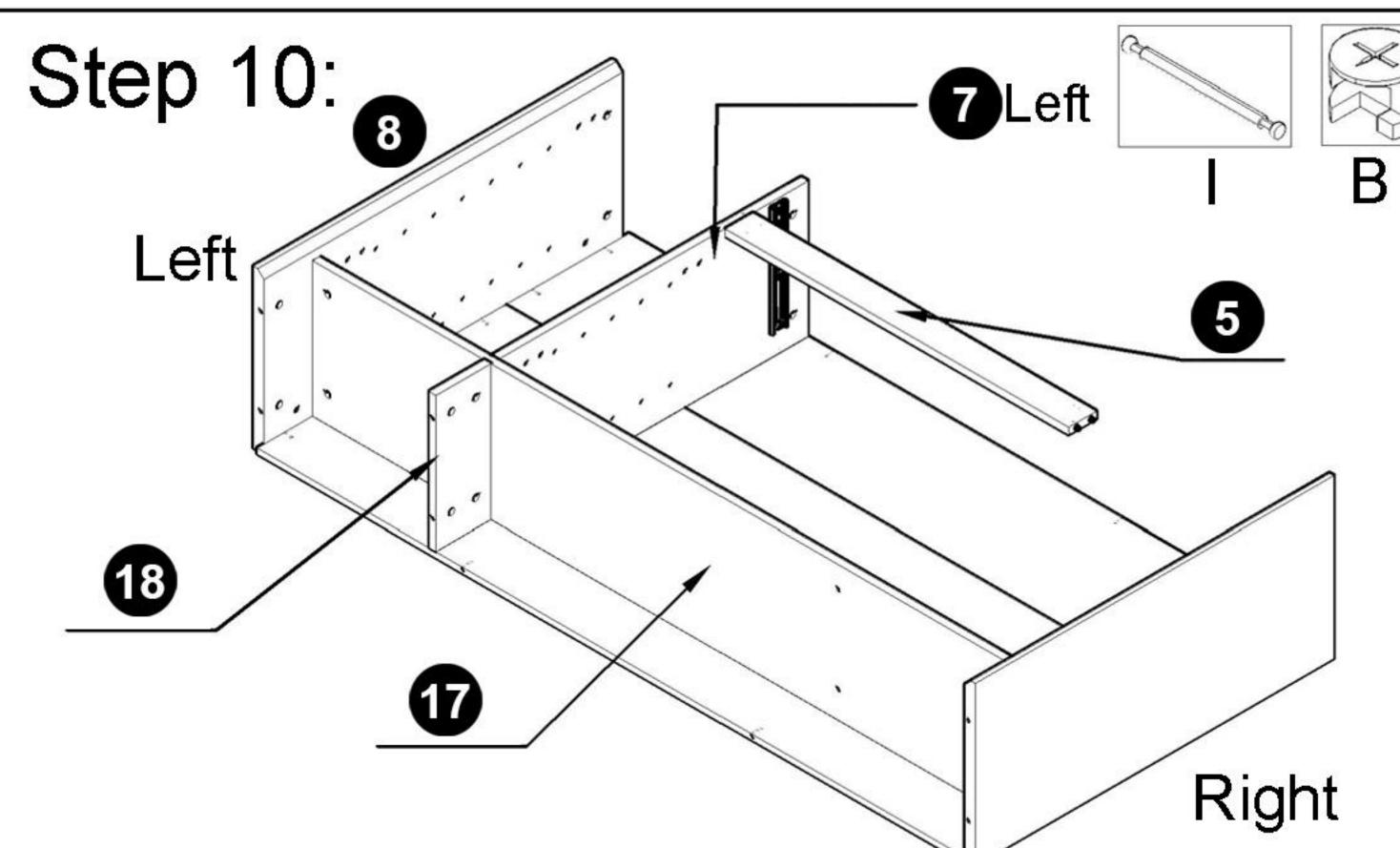
Align panels 18, 17, and 7 (left side) with their corresponding holes and connect them using I. Tighten the connections by using B. Then, align panel 5 with 7 (left side) at their corresponding holes and connect them and tighten the connections by using B
