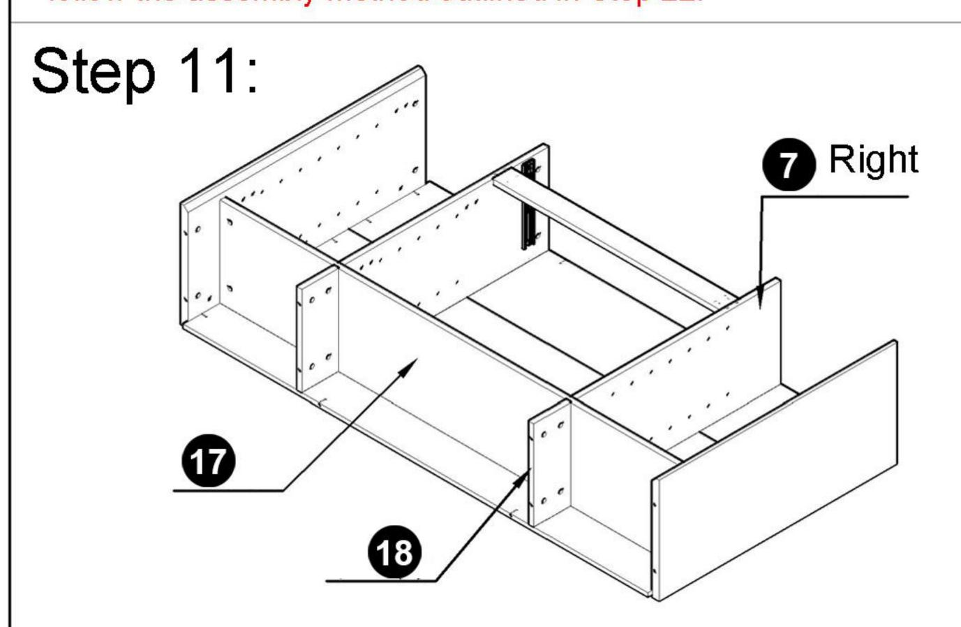
Repeat the previous step for 7 (right side). Align it with the corresponding holes of the other panels, connect using I, and secure with B.
