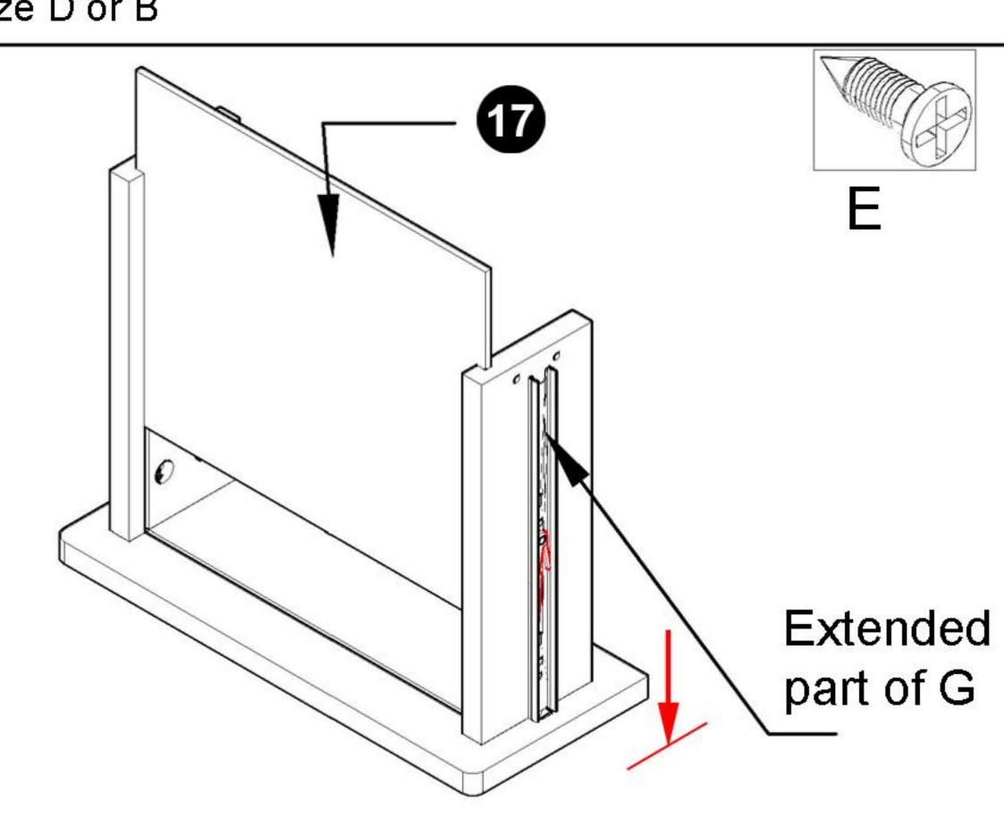
Insert panel 17 as indicated by the arrow. Position the extended part of G on the outside of both panel 14 pieces. Ensure the stopper side of G rests against panel 13
