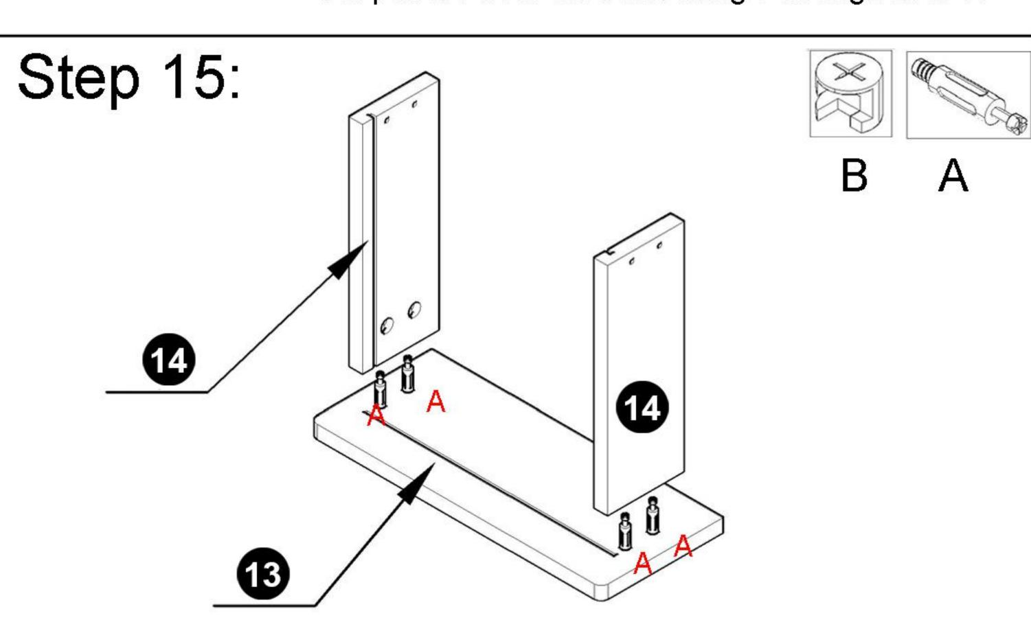
Note: The grooves on panel 13 must align with the grooves on panel 14, and secure all joints with B
