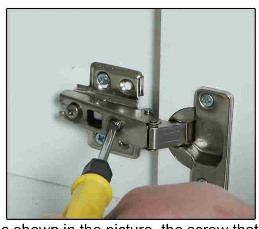
As shown in the picture, the screw that the screwdriver points to is used to adjust the door panel to move left and right, and turning it clockwise is to adjust the door panel to move toward the center.
