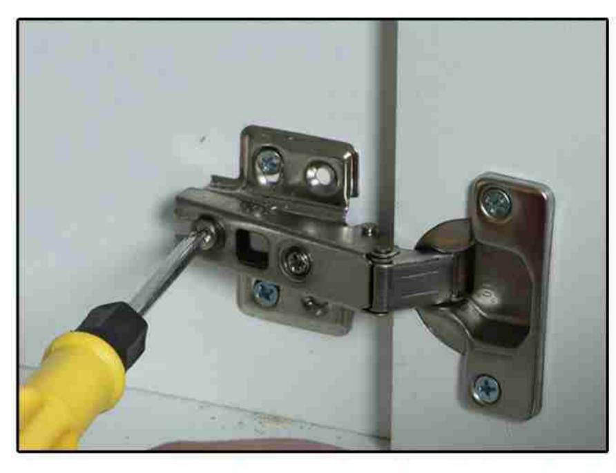
As shown in the figure, loosen the screw that the screwdriver points to, push the door panel in or pull it out, and then tighten it to solve the above problem.
