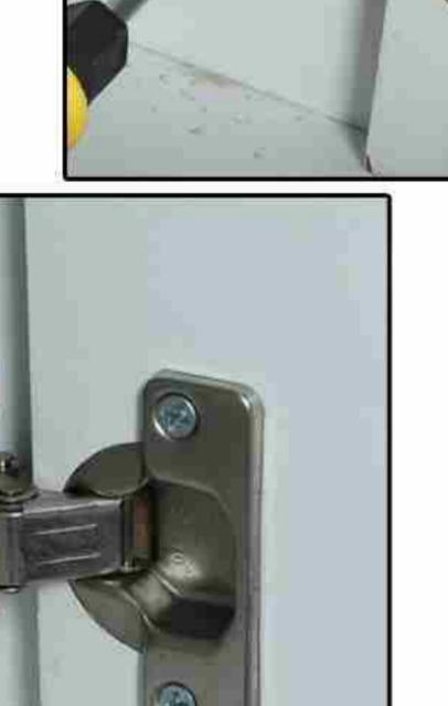
As shown in the figure, loosen the screw that the screwdriver points to, push the lower door panel and hinge upward, and then tighten the screw. Push the upper door panel and hinge downward, and then tighten the screw.
