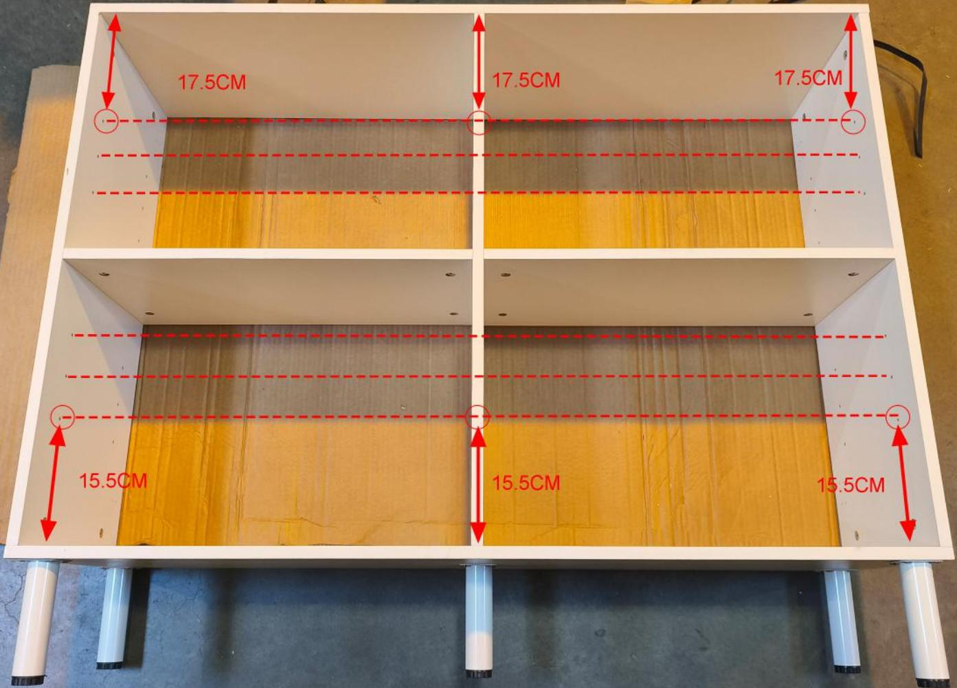
Check if the pre-drilled holes on the side panels are level. You can also measure the distance from the holes to the top panel. If they are uneven, try flipping or repositioning the panel. Note: The distance from the pre-drilled holes to the top panel is greater than the distance to the bottom panel.
