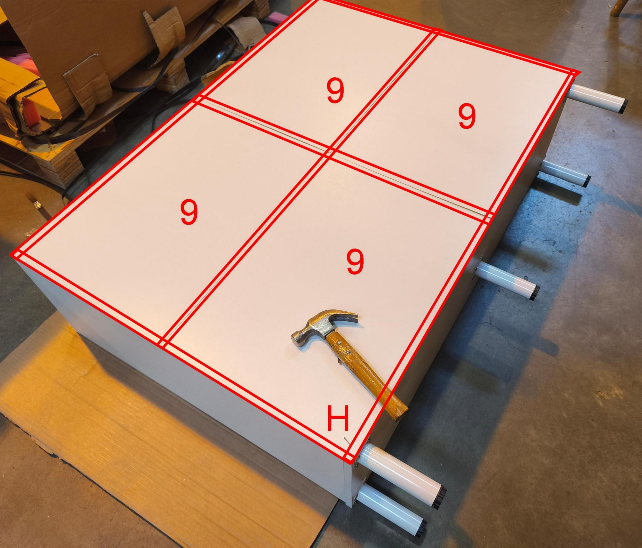
Place 9 (the back panel) in the correct position, fully covering the back side of the cabinet. Make sure to leave enough space along the edges for proper fastening by H. 9 x 4 should be installed using the same procedure. (Hammer not included.)
