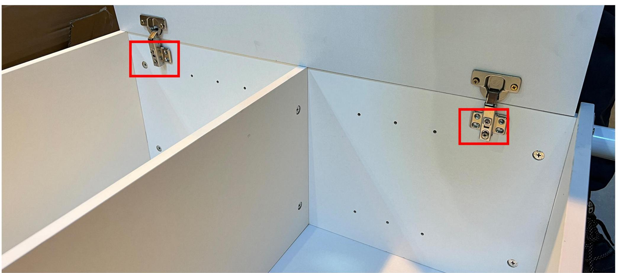
Gently flip the cabinet so the back is on the floor. The 4 small hole groups (4 per group) should face up. Attach doors 8. Use G to secure the other side of B.
