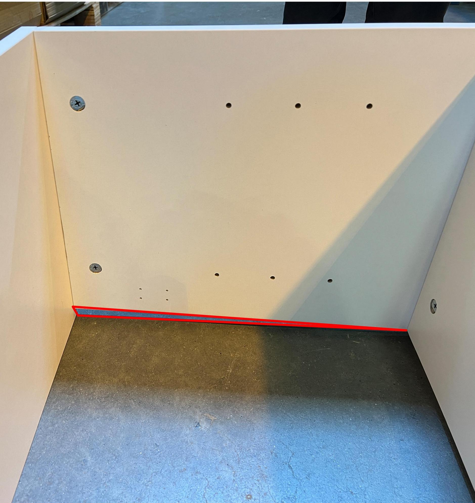
Inspect the Top for gaps. If none are visible, verify that all panels are oriented correctly.
