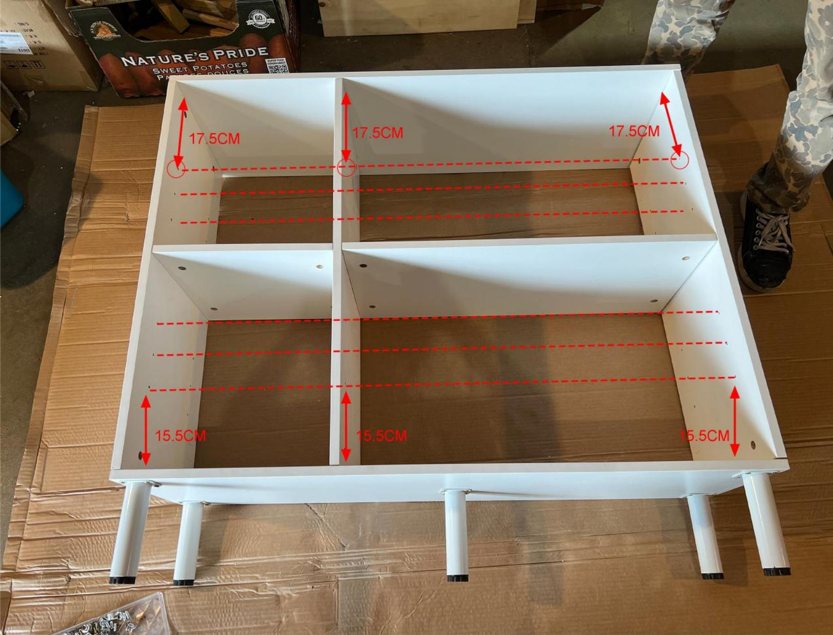
Check if the pre-drilled holes on the side panels are level. You can also measure the distance from the holes to the top panel. If they are uneven, try flipping or repositioning the panel. Note: The distance from the pre-drilled holes to the top panel is greater than the distance to the bottom panel.
