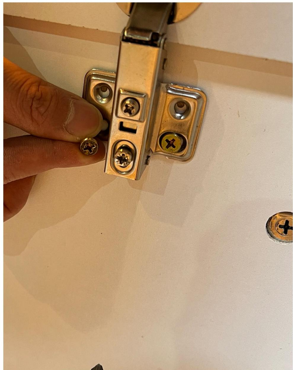
Install the two back screws first. Don't tighten yet — leave space to adjust. When all is correct, add and tighten all screws. You can adjust the door's height slightly—aim for even spacing rather than following the pre-drilled holes exactly.
