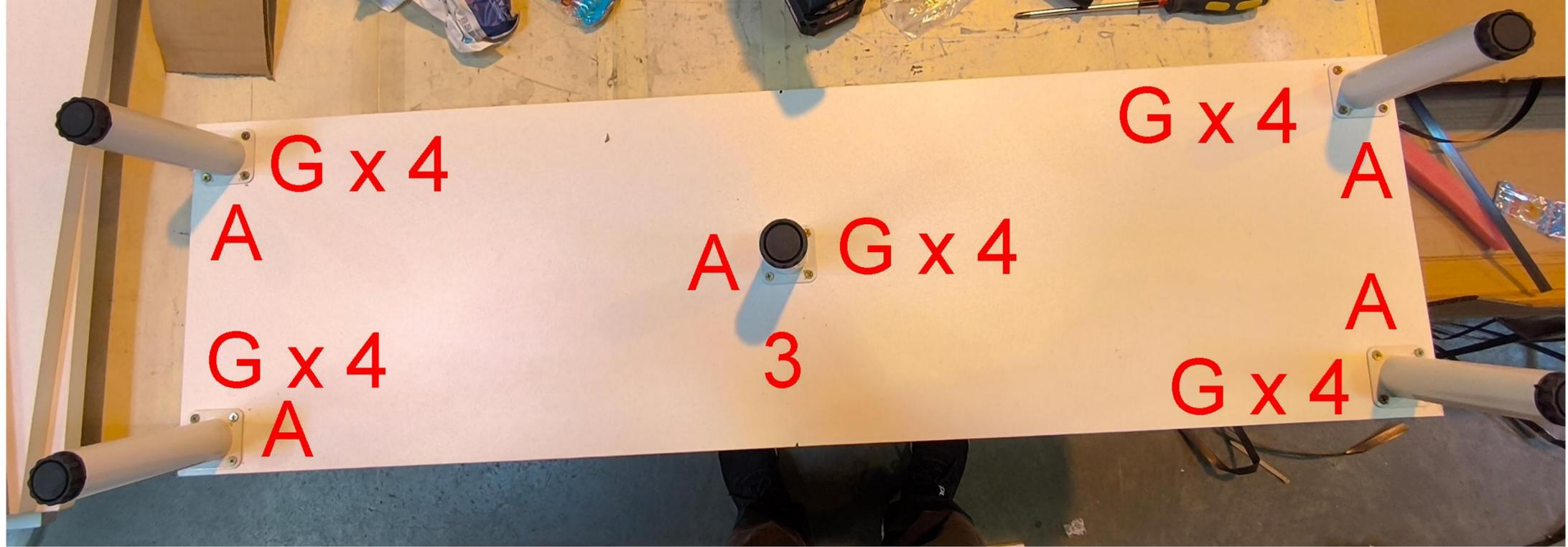
Use part G to fix part A under panel 3. There are no holes, so you need to screw it in yourself. Place A where you want it. A drill is recommended (not included).
