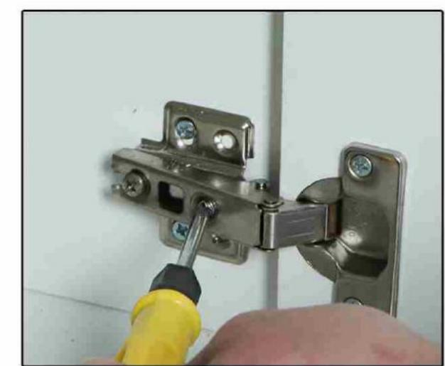
As shown in the picture, the screw that the screwdriver points to is used to adjust the door panel to move left and right, and turning it clockwise is to adjust the door panel to move toward the center.
